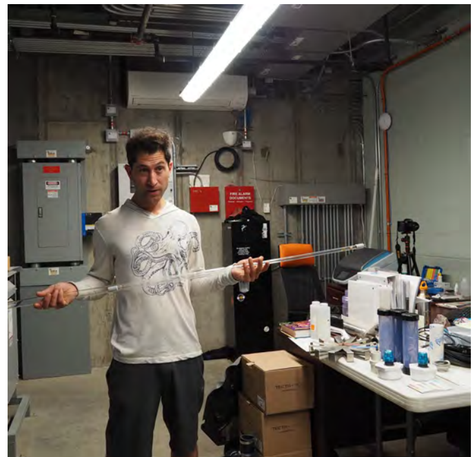
Thin long tube is a UV light tube for water purification (from IE tour in November)
